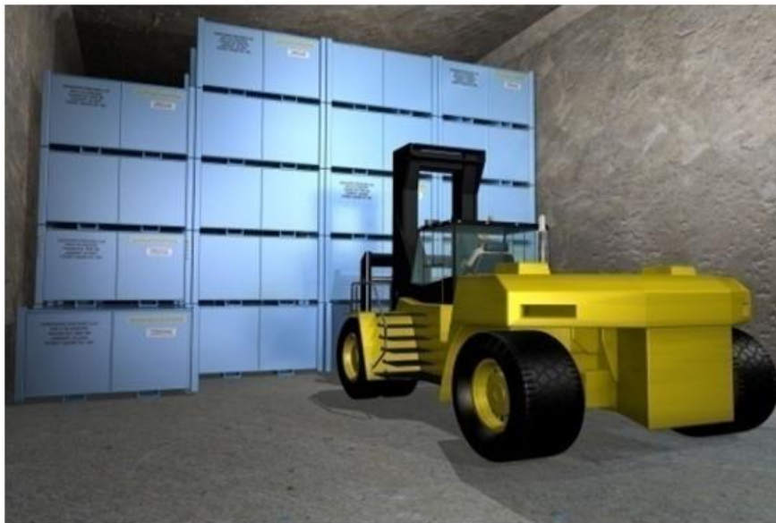
Figure 5.3: Illustration of (a) underground layout and (b) emplacement of LLW packages. Wastes are emplaced in 31 rooms in 2 panels. Rooms are 250 m long, 7 m x 8.5 m wide.
